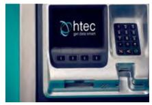
Outdoor Payment Terminals allow retailers to serve fuel 24/7 and at unmanned sites. They can be integrated onto petrol pumps or used independently to manage payment at multiple pumps and are often used at marinas, truck stops and airfields as well as on the forecourt.
